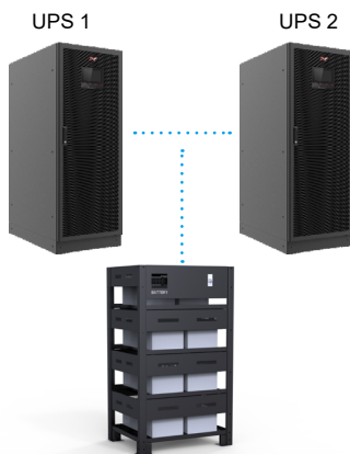
Common battery bank
